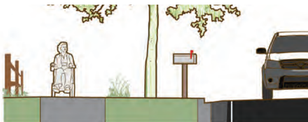
Figure 4-15. Sidewalks on roads with curbs may feature an unpaved or paved furnishing zone separation (left), or may be constructed with curb and gutter, immediately adjacent to the roadway (right). Offering separation from the roadway is preferred in most areas for user comfort and design flexibility at intersections.
