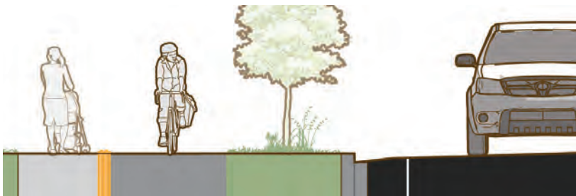
Figure 4-20. Separation from the sidewalk is valuable for reducing unwanted pedestrian encroachment into the bike lane. The use of physical separation with vertical elements, unpaved separation, or detectable edges may be more effective than visual delineation.
