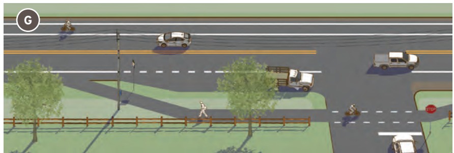
Figure 3-6. In this scenario, the shoulder is designated as a separated bike lane. Bicyclists are shifted laterally away from the roadway and separated from the travel or turn lanes by an unpaved buffer space.
