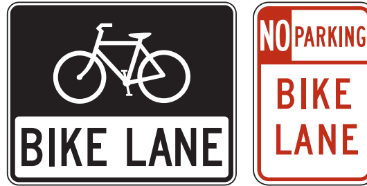
Figure 3-9. An optional R3-17 Bike Lane sign may be used to supplement bike lane markings. An R7-9 sign may be used if parked vehicles frequently block the bike lane.
