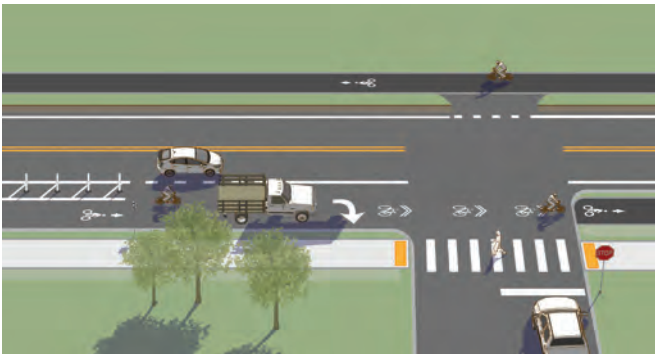
Figure 4-22. A variety of design treatments exist depending on the roadway configuration, available curb-to-curb width, traffic volumes and desire to provided a dedicated turn lane. All designs should strive to reduce speeds of turning vehicles, remind users of bicycle priority, and clarify user positioning up to and through the intersection.
