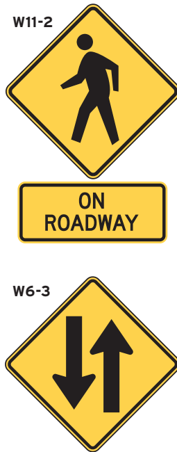
Figure 2-3. Pair a W11-1, W1-2, or W11-15 warning sign with a custom legend plaque to inform road users that shared use by pedestrians and/or bicyclists might occur.
