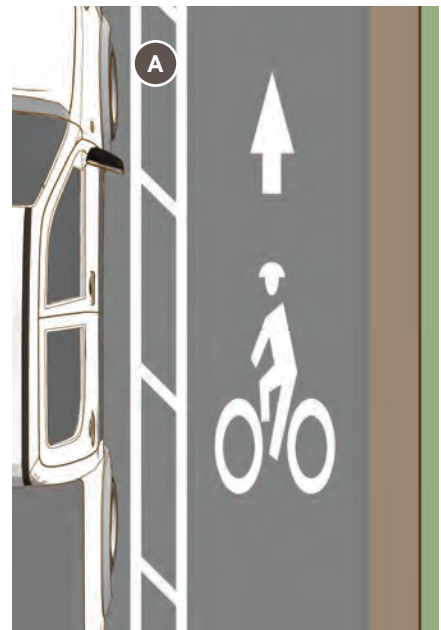
Figure 3-8. Helmeted bicyclist symbol inside a bike lane with a painted buffer area.
