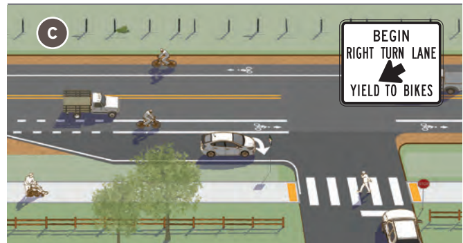
Figure 3-10. A variety of design treatments exist depending on the roadway configuration, available curb-to-curb width, traffic volumes and desire to provided a dedicated turn lane. All designs should strive to reduce speeds of turning vehicles, remind users of bicycle priority, and clarify user positioning approaching and through the intersection. Common signs at intersections include R4-4 Begin Right Turn Lane Yield to Bikes and a modified R10-15 Turning Vehicles Yield to Bikes sign. (1)
