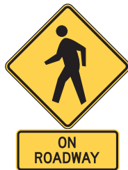
Figure 5-8. A W11-2 warning sign may be paired with a legend plaque to inform road users that shared use by pedestrians and/or bicyclists might occur.
